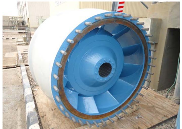
Pictured (before, left, and after, above): A recent refurbishment project, a Cold Water Pump at the largest Power Plant in Karachi, Pakistan.
